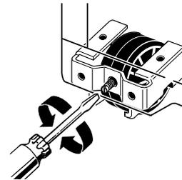
6. If the doors do not close on their own, you will need to raise the front of the refrigerator so it is slightly higher than the back. To do this, turn both leveling screws clockwise  $\frac{1}{2}$  turn. **IMPORTANT:** Be sure to turn both screws an equal amount or the refrigerator will no longer be level side to side.
